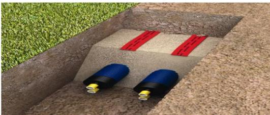
A Microflex pipe buried at a depth of no less than 50 cm and no more than 6 metres can bear a load of up to 60 tonnes. Placement must be performed in compliance with the prevailing ATV-DVWK-A127 guidelines for buried pipes.
