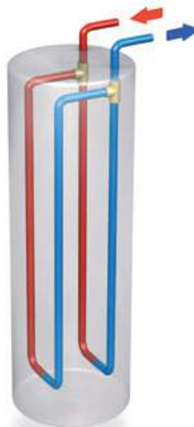
Fig. 56: U probe pipe laying
