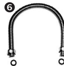
**6** Now the tube is ready to be mounted in its place. Shape it into the desired form and use the appropriate gaskets **(6)**.
