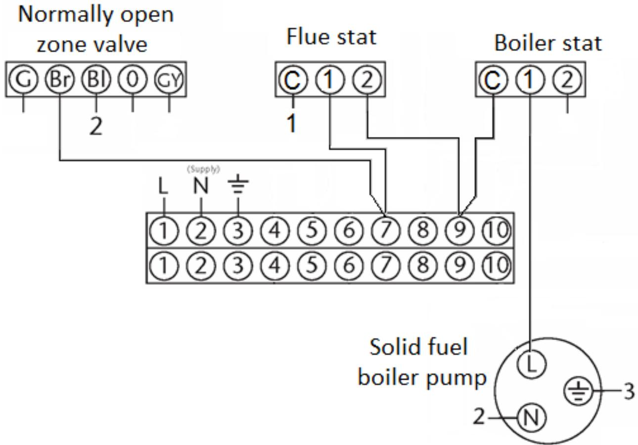
We recommend that the flue thermostat is set to approximately 50°C, the boiler thermostat is set to 60°C and the heat store control thermostat is set to 70°C. As is usual with this type of installation some degree of fine tuning will be required.
